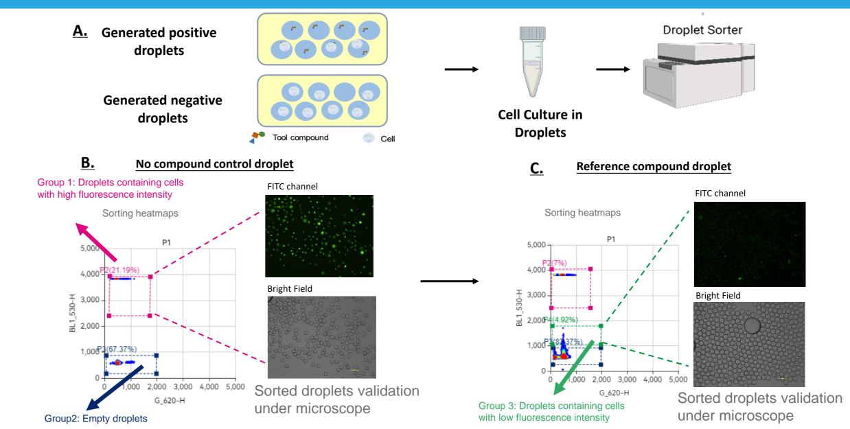
On-bead DEL tool compound sorting test of TPD assay in droplets (A). Illustration of workflow of tool compound beads sorting. The fused protein with GFP degradation after reference compound treatment (C) with fluorescence signal decrease were observed compared with control (B) group. The cells fluorescence signal in droplets were detected using droplet sorter with high sorting
